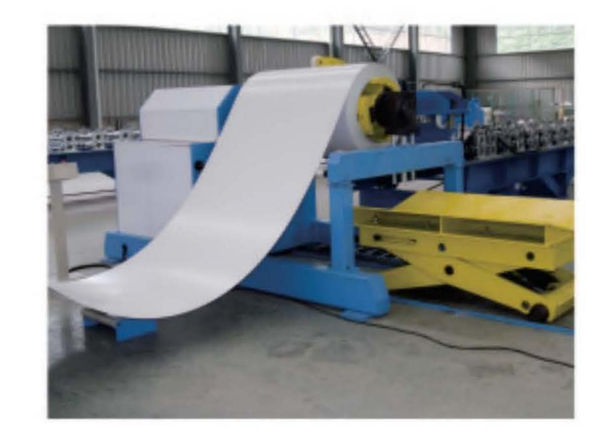
10 tons automatic decoiler with coil car
